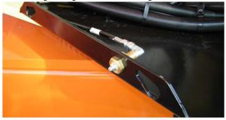
Lube Point(s) - 1 Grease Fittings Capacity - A/R Lube - MPG
