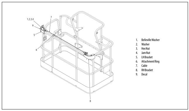
Figure 6-3. Bolt-On External Fall Arrest System
