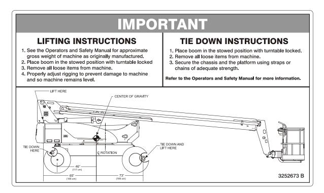
Figure 4-5. Lifting and Tie Down Chart
