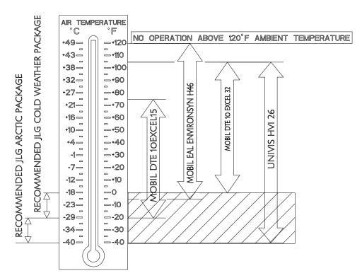
Figure 7-1. Hydraulic Oil Specification - Sheet 1 of 2
