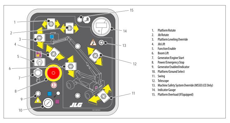
Figure 3-1. Ground Control Station
