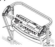
Reattach magnetic end of cable to bracket if it becomes disconnected.
