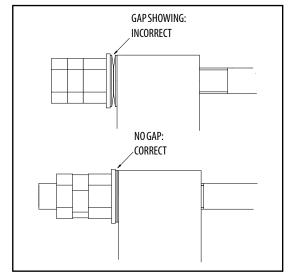
Figure 6-2. Bolt-On External Fall Arrest Cable Tension
