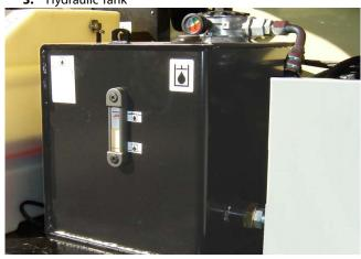
Lube Point(s) - Fill Cap Capacity - 15.9 gal. system (56.7L) 12.4 gal. (46.9 L) to Full Mark
